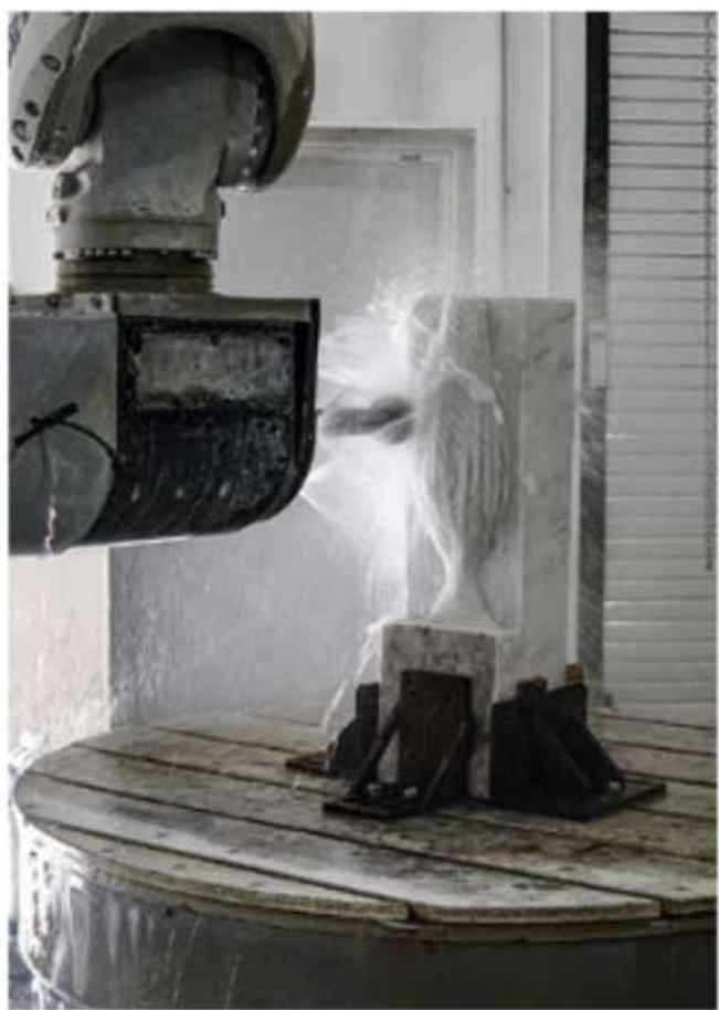
The RIPPLE pieces feature fluid forms and undulating surfaces that are milled by 7-Axis robots
