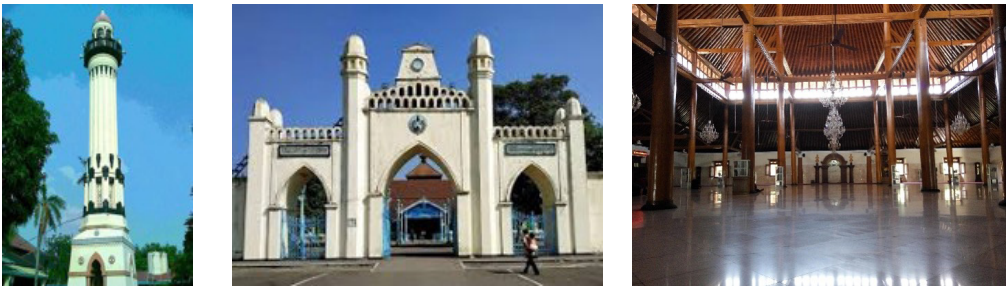
Figure 1. Passive tropical design features of the Masjid Agung Keraton Surakarta, illustrating the tajug roof and permeable spatial configuration that support natural ventilation, spatial openness, and socio-religious inclusivity.
