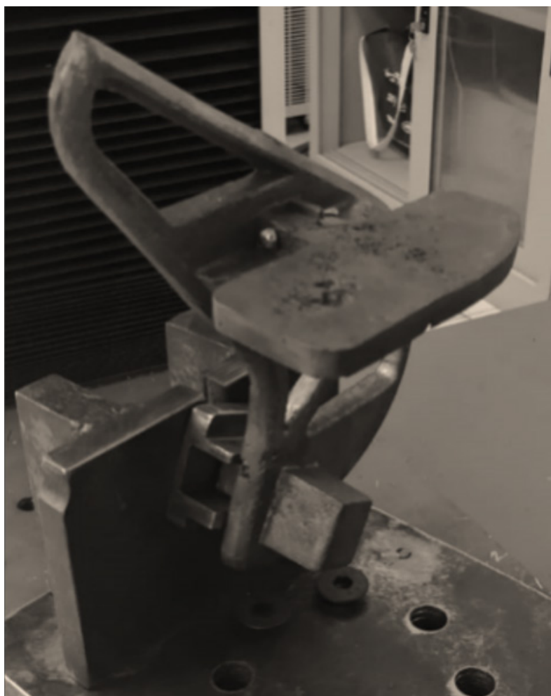
Figure 8. P.Jacq™ prepared for breaking load analysis at SIRIM
