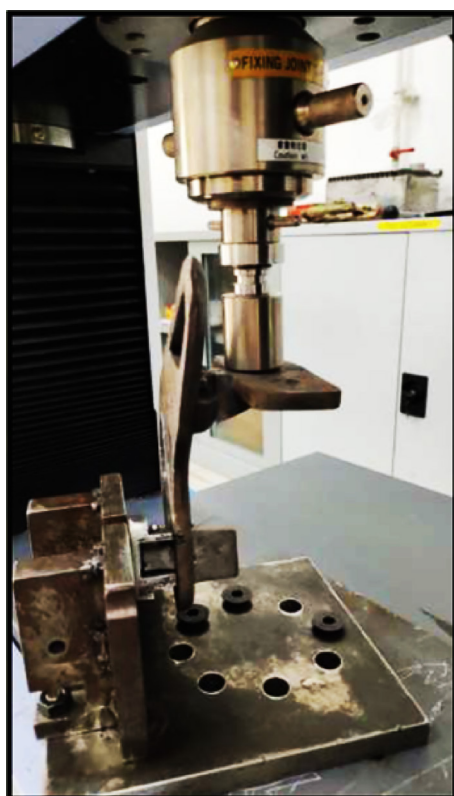
Figure 9. Breaking load test on prototype
