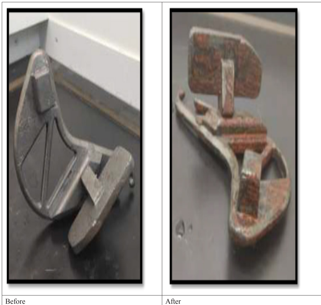
Figure 11. The sample before and after the salt spray exposure
