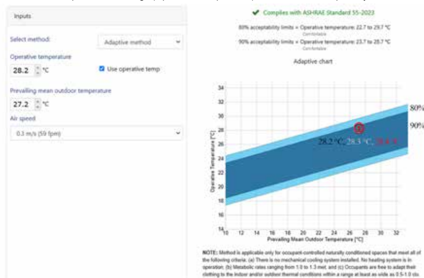
Figure 8: Thermal Comfort Temperature Readings (Operative Temperature) Based on the Acceptability Limits of ASHRAE Standard 55
