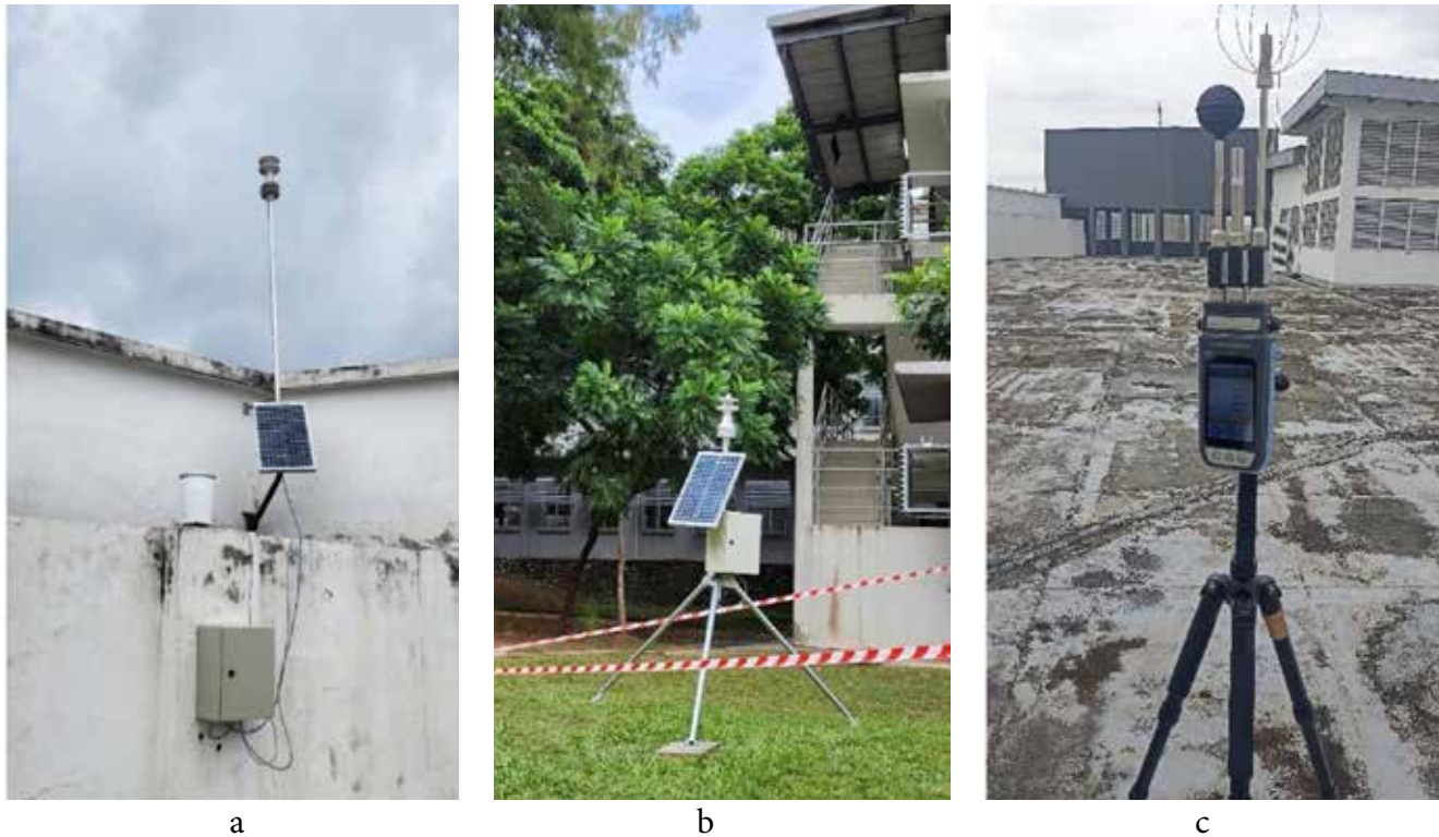
Figure 3: (a) Delta Ohm Meteo Compact Station HDMCS-200 Set Permanently on the Rooftop of A 5-Storey Building. (b) The Movable Delta Ohm Meteo Compact Station HDMCS-200 Is in the Investigated Outdoor Learning Space. (c) Portable Delta Ohm HD32.3TC Data Logger Setup Adjacent to the Respondent.
